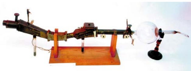
Fig. 9 Aston's third mass spectrograph, now in the the Museum of the Cavendish Laboratory. The discharge tube is on the right. The white discs are for adjusting the widths of the slits S_1 and S_2 . The magnet, not shown, acts over the region of the tube in the left-hand wooden support. The photographic plate is placed in the focus plane just before the left end of the tube to record the spectra. The overall length of the instrument, excluding the discharge tube, is 105 cm.
